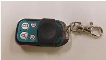
The Wi-Fi / RF models are provided with a 4 button pre-programmed hand held (key fob) remote. The “A” button controls ON/OFF power to the fan. The “B” button controls LOW/HIGH speed. C & D are not in use. You may use a 433MHz frequency remote as an alternate remote. To program follow the instructions below.
