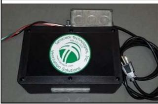
**IMPORTANT:** Perform these tasks before the fan has been installed. To connect the Wi-Fi receivers to the home network, disconnect the control box from the fan and provide power to the control box ONLY.
