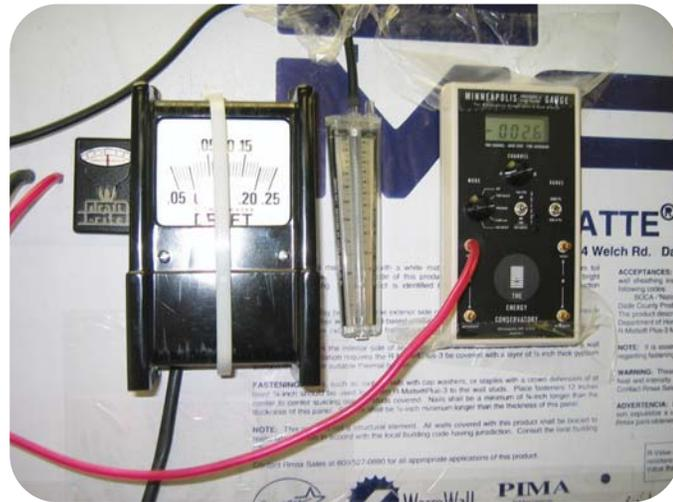
Pressure measurements were made using an inexpensive digital manometer.
