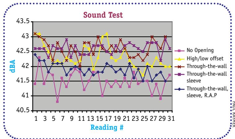
Figure 2. This graph shows the comparative sound attenuating performance of four pressure approaches to a baseline noise level with no openings in the walls of the test room.
