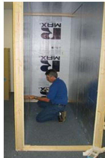
Figure 95. Return Air Flow Test Chamber
